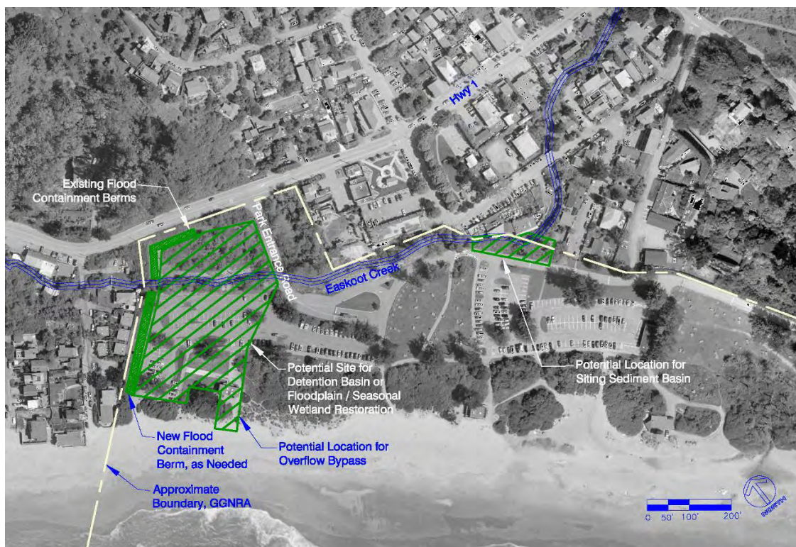
Figure 6 - Conceptual Plan for wetland restoration and sediment detention basin completed by Mike Love & Associates (one possible alternative)
